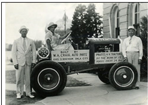
B. A. Pratt (right) with a tractor he designed from used auto parts to help farmers survive the depression.
